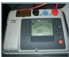
Insulation control with Megger measuring device
